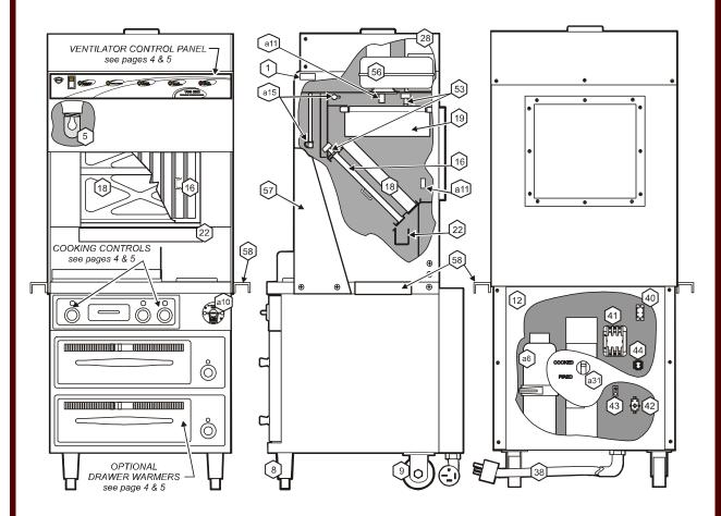
Fig. 1 Ventilator Section Operating Features & Controls
